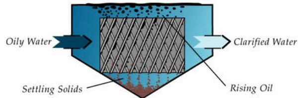
than water, they (oil) will rise up the coalescing plate. As the oil droplets rise up the plate they will coalesce or come together with other droplets, creating progressively larger droplets. Once the droplet size is sufficient or the droplet reaches the top of the media plate the droplet pulls away from the plate and rises to the water surface. To some degree, the solids replicate this process in reverse (settling).
