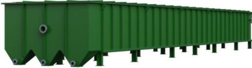
The API is the oldest of the modern gravity separator designs. Built to API 421 criteria its performance is <100mg/L, 150-micron free non-emulsified oil droplets. This design provides the solution for heavy solids and oil removal applications.
