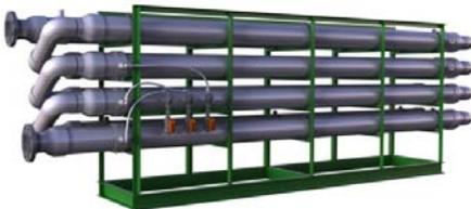
The STAX systems are a pipe flocculator design that provides multiple-chemical reaction contact in a compact, small footprint design without moving parts, wearing components and no need for power. The STAX design uses water turbulence induced by a spiral piping network to mix chemical products into a wastestream.
