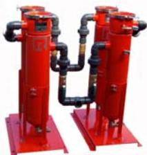
Bag filtration has become a standard technology for water treatment and we provide it as required in many projects. The filters can be provided in multiples, singles in parallel or sequential or duty/standby orientation with isolation and with switching automation and/or pressure monitoring.
