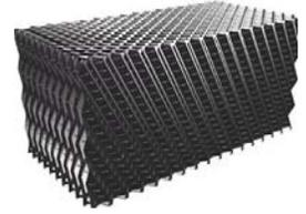
Flopak is a standard feature of our high performance separators and is also offered for replacement or retrofitting of existing tanks to improve performance and increase flow rates. Removal efficiencies have been as low as <1 mg/L down to non-detect. Typical, regular performance is in the 3-10 mg/L depending on wastestream characteristics.
